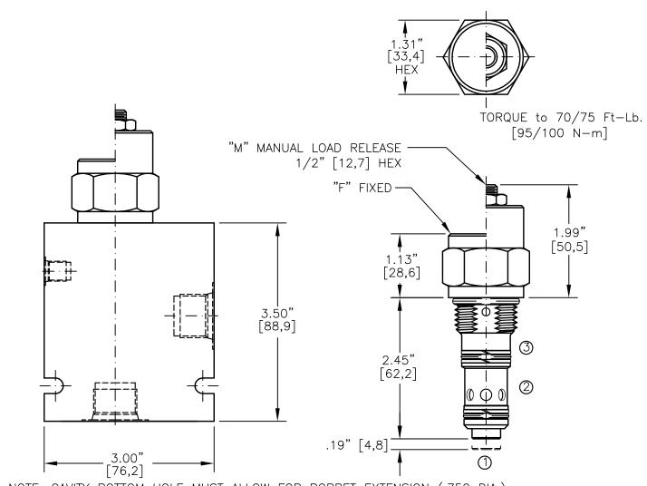
NOTE: CAVITY BOTTOM HOLE MUST ALLOW FOR POPPET EXTENSION (.750 DIA.). FOR ALUMINUM OR STEEL VALVE HOUSING CONFIGURATIONS SEE PAGE 0-023-1.
